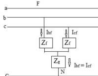
Fig 6: Double Line-to-Ground Fault
