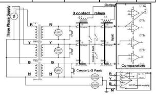
Fig 11(a): Schematic diagram of 3 phase fault analysis
