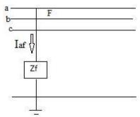
Fig 4: Single Line-to-Ground Fault
