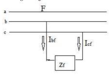
Fig 5: Line-to-Line Fault
