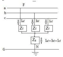
Fig 7: Three phase Fault
