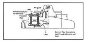
Fig 3: Lightning Arrester Unit with ZnO
